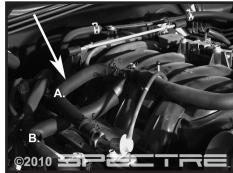
Step 5 Remove breather hose A. from the factory T fitting.
