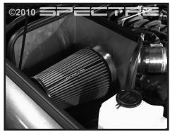
Step 17 Install the air filter onto the velocity stack. Tighten clamp fully.
