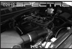
Step 2 Lift and remove engine cover.
